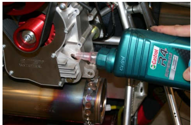
Oil filling location
