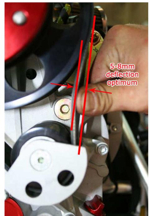
**N.B. Do not over-tighten belt – This may lead to premature bearing failure and reduction in available thrust.**
