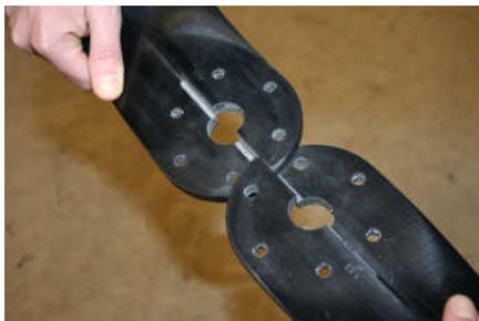
Propeller halves slide together
