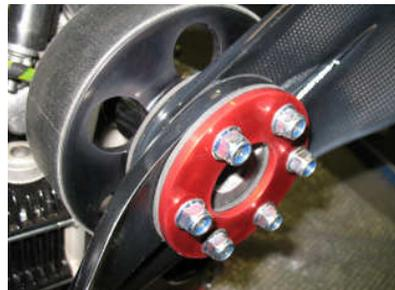
6 nut propeller mounting
