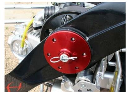
Quick release propeller mounting
